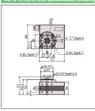
**RCP2-RTC/RTCL Combination Drawing**
